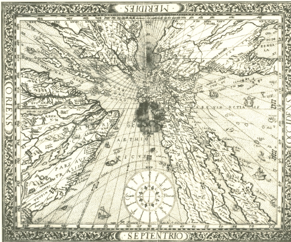
World map by Franz Ritter, 1610. The gnomonic projection imagines the earth projected onto a tangent plane and allows any great circle to be shown as a straight line. Ritter had produced an air-age map long before its time. (From the Franco Novacco Collection, the Newberry Library, through whose courtesy it is used.)
