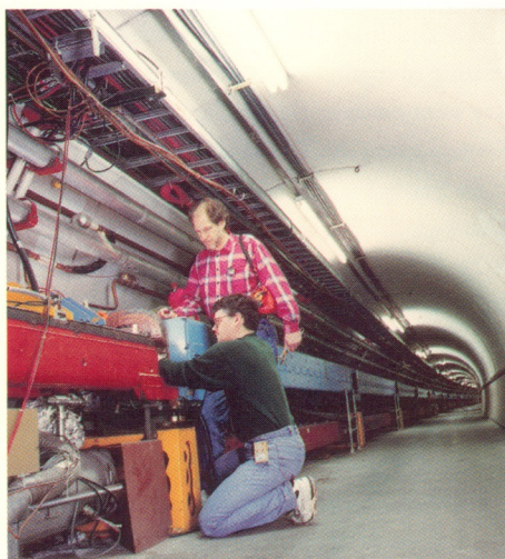
Engineers work on the Main Ring accelerator. This is an interior view of the Tevatron accelerator, which is made up of 1,000 superconducting magnets. (Image 95-341)
